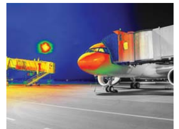
Luminance distribution and horizontal illuminance measurement on the aircraft parking area
