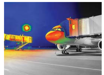
Luminance distribution and horizontal illuminance measurement on the aircraft parking area
