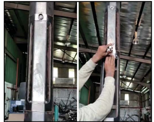
Sliding Service Door c/w Special Locking System
