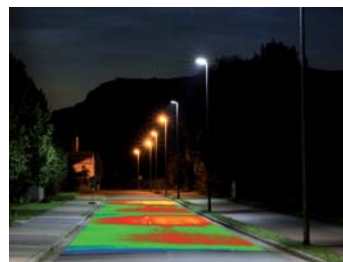
Determination of glare according to the TI method
